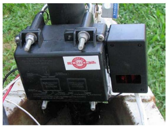
Figure 8. Battery box on left, Solar Float Charger attached on right.
